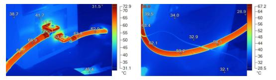
Maximum temperature observed 58.5°C, using the thermocouple method and around 72.5°C, using the thermography method. Heat Rise as per standard should have been 45°C. Maximum recorded Heat rise is 40.8°C. (Calculation = 72.5°C using thermography minus 31.7°C Ambient).
