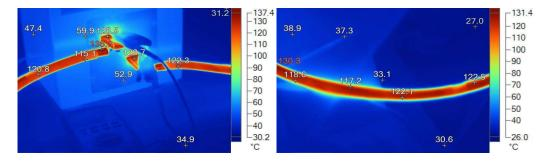
Maximum temperature observed 126.7°C, using the thermocouple method and around 136.8°C, using the thermography method. Heat Rise as per standard should have been 140°C. Maximum recorded Heat rise is 103.3°C. (Calculation = 136.8°C using thermography minus 33.5°C Ambient).
